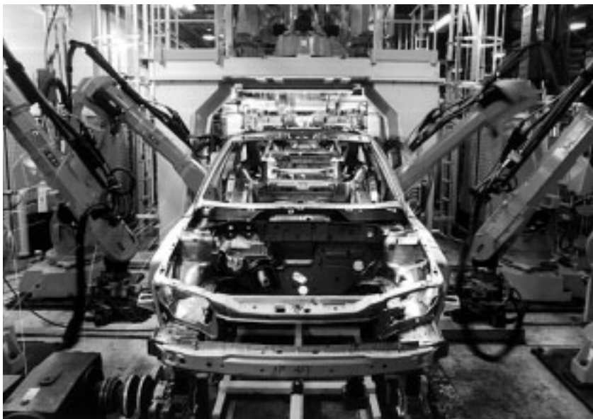
Robotic welding of the Vectra body.
