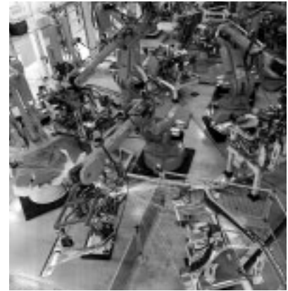
Robotic spot welding of the Vectra wheel arch.
