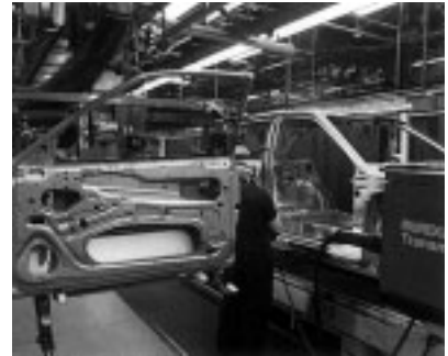
The body in white line where the sub-assemblies are added to form the complete body.
