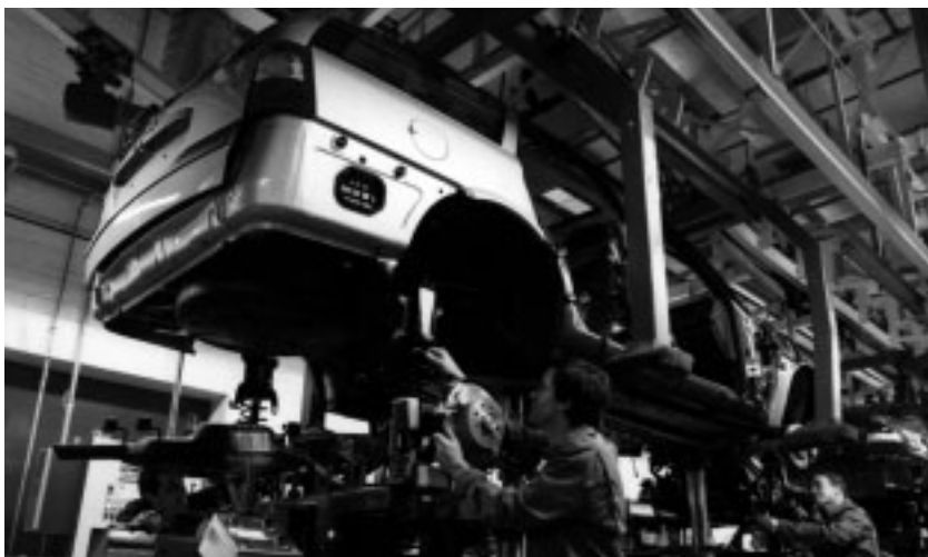
The 'Marriage' of a Vectra Estate body and its mechanical units.
