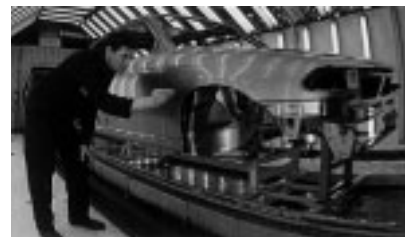
Experienced operators use sight and touch to detect any imperfections.
