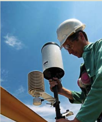
Measurement of air quality at Rustenburg Platinum Mines' Waterval Smelter
